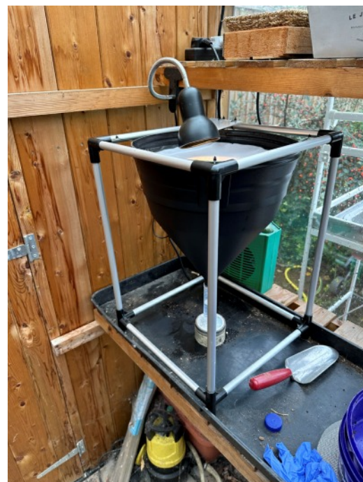
Fig. 1. Berlese Funnel set up in the greenhouse.
